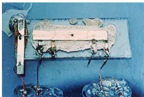
Jack Kilby 's original integrated circuit
